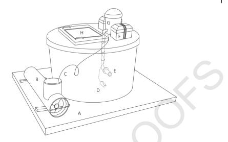
**Figure 26.1** Transport tank for live fish. (A) Wooden, or plastic, pallet; (B) Stainless steel cylinder to hold oxygen cylinder (inside); (C) Airline tubing, connected to pressure regulator, in turn connected to oxygen cylinder; (D) Air stone (inside the tank); (E) 12 Volt bilge pump; (F) 12 Volt dry-cell battery; (G) Filter unit (usually laminated cartridge paper and one mesh bag with activated carbon inside); (H) Inspection and access window.
