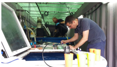
FIGURE 9 Temperature, pH, oxygen saturation rate and ammonia concentration were tested approximately every 4 h on all transports by road or water. Effluent from protein skimmers was also dumped whenever required, during water quality checks [Color figure can be viewed at wileyonlinelibrary.com ]
