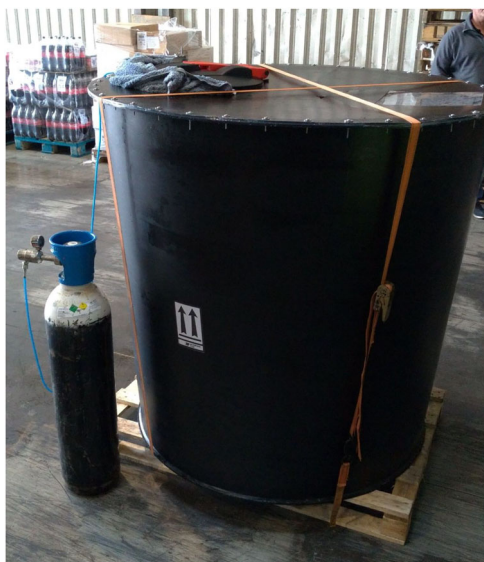
FIGURE 8 500 L, 120 cm wide and 120 cm high tank, used to move 100 Scomber scombrus from Peniche (Portugal) to Montréal (Canada), via a Lisbon to Toronto direct flight
