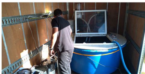
FIGURE 24 600 Sardina pilchardus which travelled inside a 1600 L tank from La Ciotat (France) to Olhão (Portugal) over 19 h. Note the fully operational foam fractionator on the left side of the tank [Color figure can be viewed at wileyonlinelibrary.com ]
