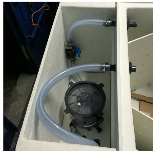
FIGURE 7 Custom-built tank for moving a 125 kg Silurus glanis from Acuario de Zaragoza (Spain) to Wonders of Wildlife (Springfield, MO, USA). A cartridge filter consisting of laminated pleated paper, with 1 kg of activated carbon in the centre, was powered by a 12 V bilge pump [Color figure can be viewed at wileyonlinelibrary.com ]
