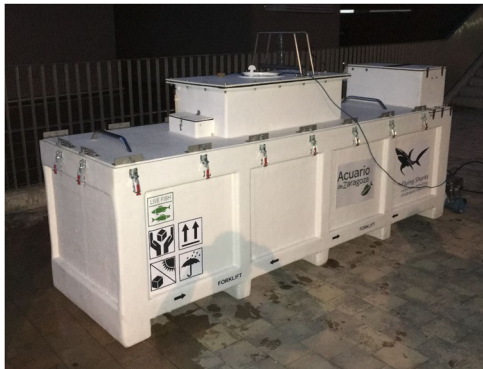
FIGURE 5 Custom-built tank for moving a 125 kg Silurus glanis from Acuario de Zaragoza (Spain) to Wonders of Wildlife (Springfield, MO, USA) via a Madrid to Chicago direct flight [Color figure can be viewed at wileyonlinelibrary.com ]
