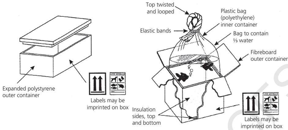
**Figure 26.2** IATA (International Air Transportation Association) Live Animal Regulation number 51, for transporting live fish inside plastic bags, which travel inside polystyrene boxes that, in turn, must travel inside a cardboard box.
